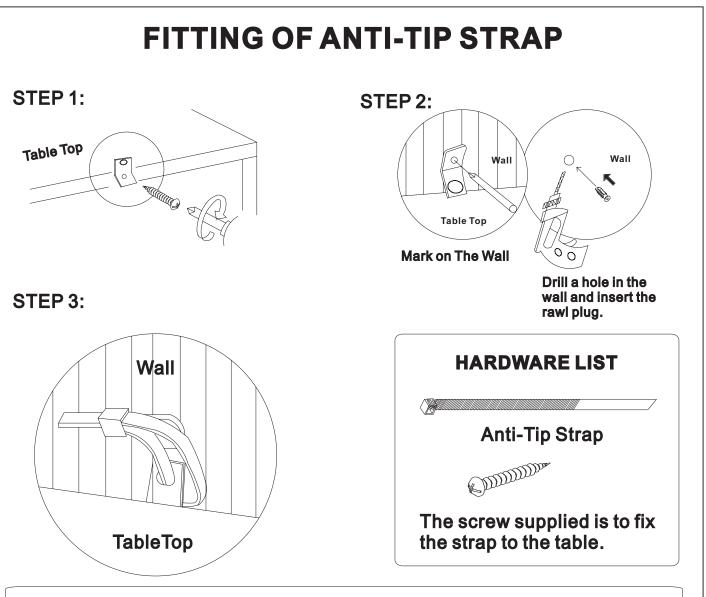
Note:Wall fixings are not supplied with this product as different wall materials require different types of fixing devices (such as Rawl plugs on brick work). You must use fixing devices suitable for the typle of wall you intend to mount this product to.
