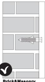
Brick&Masonry (Can use rawl plug as shown)
