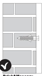
Brick&Masonry (Can use rawl plug as shown)
