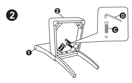
Place the screws in the holes and tighten the screws. Do not over-tighten (90% tight is sufficient)
