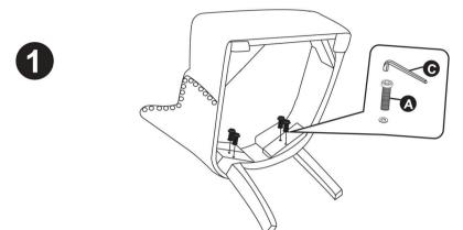
Place the screws in the holes and tighten the screws.
