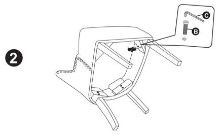
Place the screws in the holes and tighten the screws. Do not over-tighten (90% tight is sufficient)
